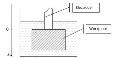
The workpiece wants to be machined up to 50 mm depth as the left side picture.
