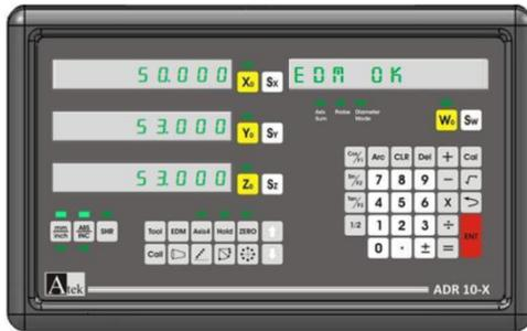
When 50 mm + 3 mm (Offset) depth value is received the relay changes its position and digital readout warns the user both by written and sounds. To exit press EDM button or enter or
