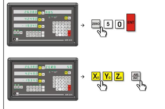
• Also the coordinate memory can be set by manuel one by one. To save the coordinate points in memory press "ZERO" button, enter the memory number and press "ENTER". To enter to X coordinate press "Sx", to enter to Y coordinate press "Ys", to enter Z coordinate press "Sx" and to enter Z coordinate press "Sw" button and enter the coordinate value by numeric buttons.
