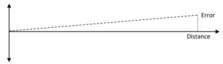
For linear error compensation only one value would be entered as "Correction Factor" to each axis. Correction Factor can be calculated according to which value is showed for 1000 mm (1 meter).
