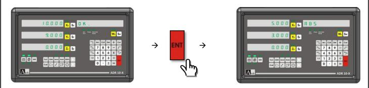
When the work pieces are moved up to make zero all axes you will find the work piece centre.
