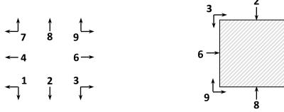
For Tool Diameter Compansation function moves the tool edge to the start point which the machining will be started. And Tan / F3 button is pressed. On work piece the machining side must be selected by numeric buttons. By
