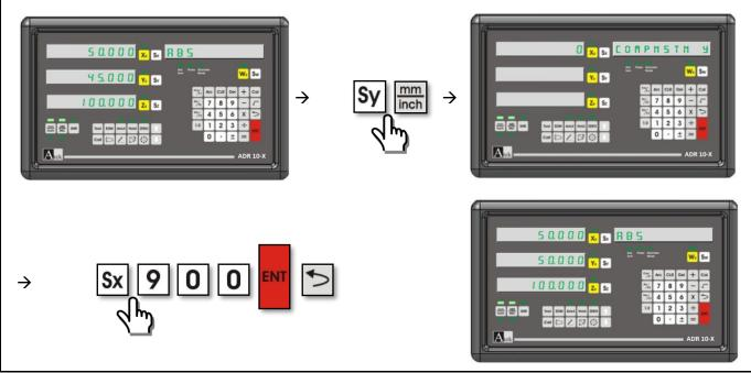
**5.2.2. Segmented Error Compansation Function:** If the scale makes errors in different dimensions this function is used for compensation. It can make compensation up to 100 point. Please select segmented option from system setting menu.
