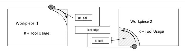
As on the work piece 1 convex would be given R+ Tool should be used. You can travel by button. After selection please press enter to save.
