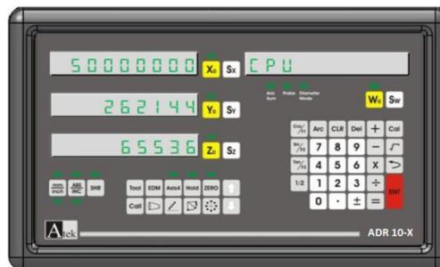
On X axis, it shows drawer speed in Hertz unit, on Y axis drawer flash memory in Byte unit, on Z axis RAM in byte unit.
