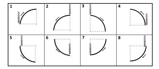
button is used to enter to the function. By button find the "Simple R." writing. Press enter and find the plane by buttons. Press enter to save. On the info screen after "TOOL PATH" writing, select one of the 8 tool ways. After writing the number as 1 to 8 press enter to save. Enter the circle Radius. Press enter to save. Enter "Maximum cutting distance and press enter. Determine if the tool diameter must be add or subtract.
