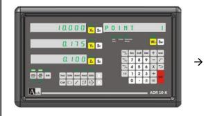
The workpiece is machined up to axis values are zero. By button the next coordinate is screened. Up to machine whole part these operations are repeated. Press button to exit.
