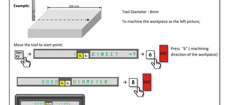
→ The work piece will be machined up to the X axis values are 100.000.
