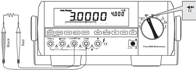
Figure 3-10. Resistance Measurement
