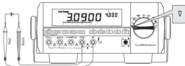
Figure 3-1. DC Voltage Measurement
