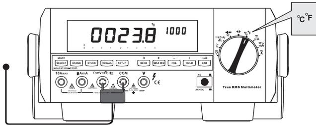
Figure 3-15. Temperature Measurement
