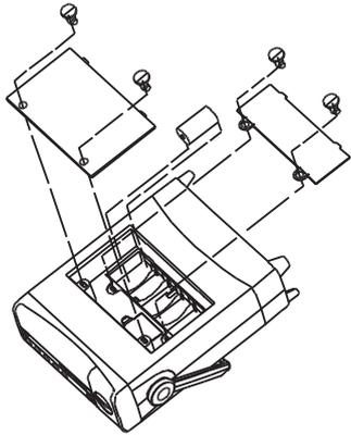
Figure 6-2. Battery Replacement
