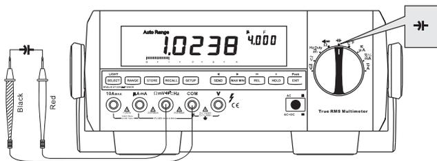
Figure 3-13. Capacitance Measurement
