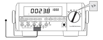
Figure 3-15. Temperature Measurement
