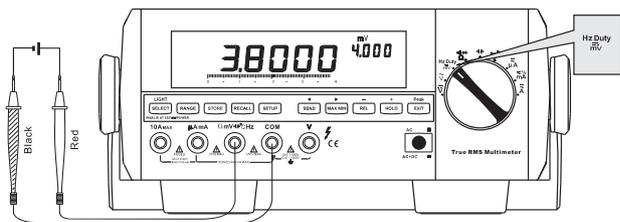
Figure 3-3. DC Millivoltage Measurement
