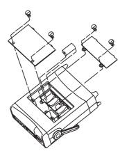
Figure 6-2. Battery Replacement
