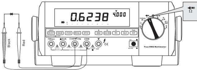
Figure 3-12. Diode Test
