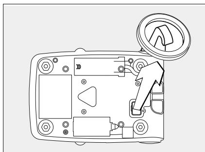
A port for a below-balance weighing hanger is located on the bottom of the balance/scale.
